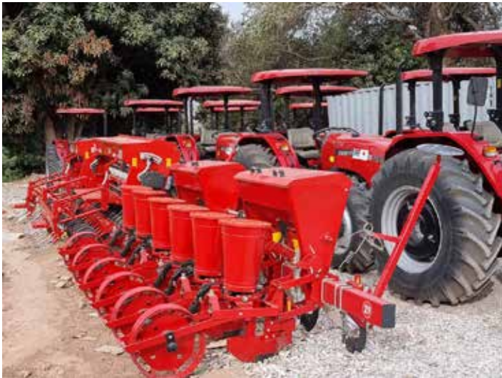
6-row seed drill (for sowing) Semoir 6 rangs (pour le semis)
